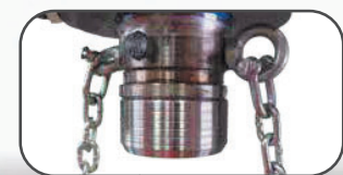
Hardened ram nose with easy change tools
