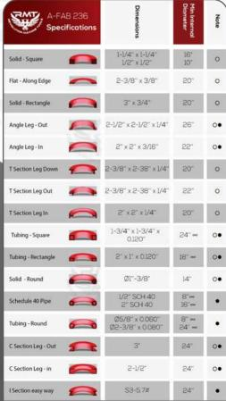
Capacity based on mild steel  $|\infty|$  be changed according to deformation o Standard Rolls  $|\bullet|$  Special Rolls |X| Special Support Rolls |A| Special Tools
