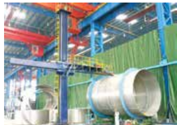
Outside Welding Machine
