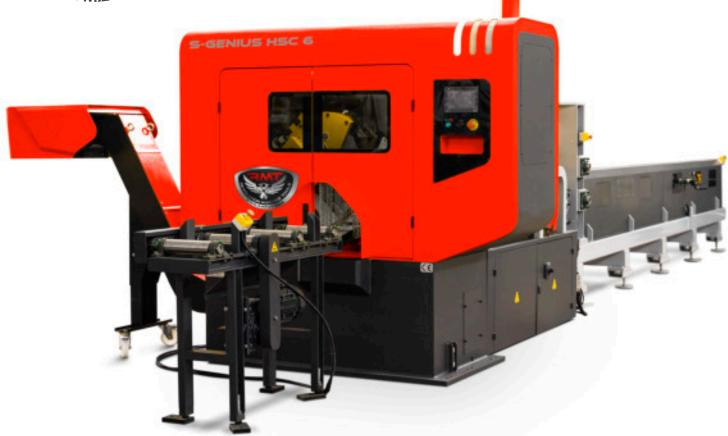
Mass production in continuous operation is done by S-GENIUS HSC Saws, when producing cut-off pieces of steel and non-ferrous metals. They are designed to be used with TCT (Carbide Tipped) circular saw blade in order to cut solid bars in high speed and excellent accuracy.
