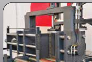
39- SERVO MOTOR FEEDING VICE 120" STROKE
