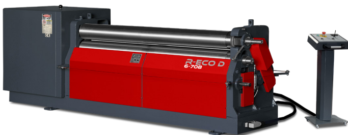
R-ECO-D Series Motorized Initial Pinch Three Roll 3' ~ 10' Bending Lengths 5.90" ~ 7.08" Top roll diameter Up 3/8" Capacity
