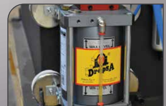
40- DROPSA AIR/ OIL CLEAN LUBRICATION SYSTEM
