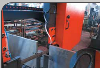
33- PROXIMITY SWITCH FOR SENSING BLADE SLIPPAGE
