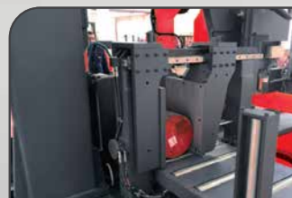
35- SERVO MOTOR FEEDING VICE 27" STROKE
