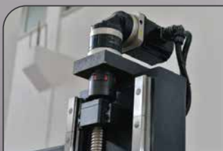
37- SERVO MOTOR DRIVEN BALLSCREW DOWNFEED SYSTEM (CNC SMART CUTTING)
