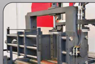
39- SERVO MOTOR FEEDING VICE 120" STROKE
