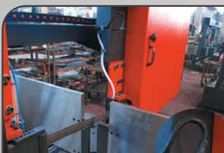
33- PROXIMITY SWITCH FOR SENSING BLADE SLIPPAGE
