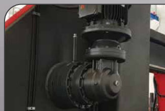
38- HEAVY DUTY PLANETARY GEARBOX
