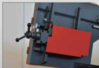
15-HYDROMECHANICAL BLADE TENSION
