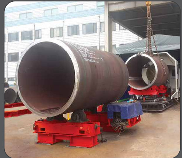
Giant Pipe Beveling
