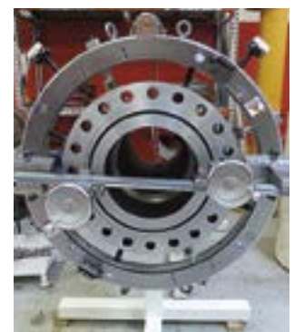
Two FFR modules performing simultaneous operations
