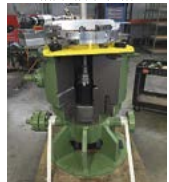
EICC Casing Cutter used for wellhead completion
