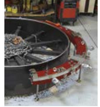
Four standard LDSF sizes cover 60-120in (DN1500-3000)
