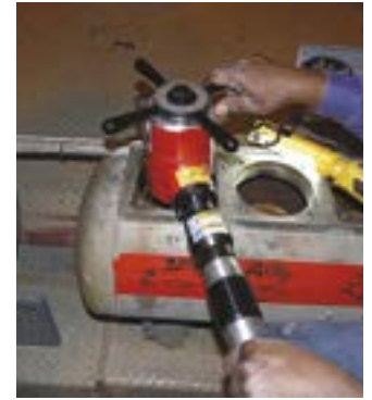
Box header beveling with SDB
