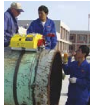
Trav-L-Cutter is designed for pipeline operations.
