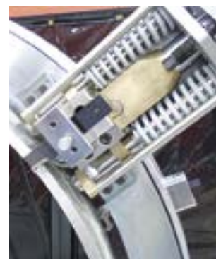
OD tracking slides follow out-of-round pipe & vessels.
