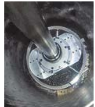
Internal cutting module lowered to cutting depth
