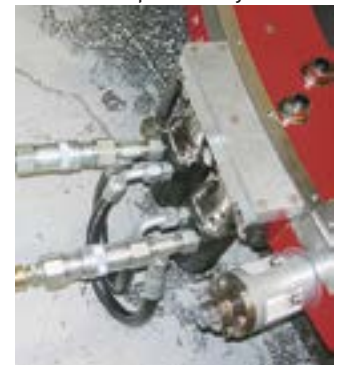
LDSF standard dual hydraulic drive motors & dual pinion housings
