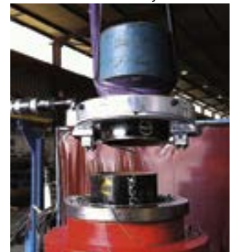
ECC can be inverted for cuts low to the wellhead
