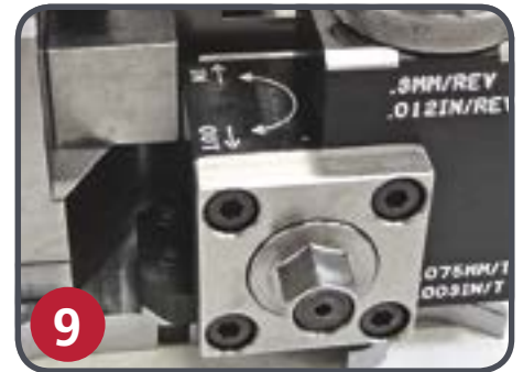
Rapid Adjust feature speeds positioning of tooling
