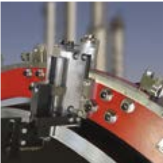
LDSF Large Diameter Split Frame for pipe & vessels
