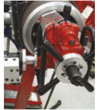
EP 424 SpeedPrep™ deluxe beveling with form tool rotating head
