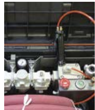
Ergonomic fingertip control with safety stop button
