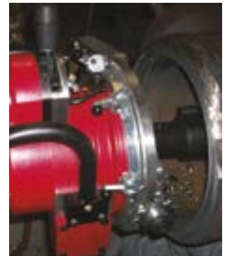
Self-centering standard mandrel
