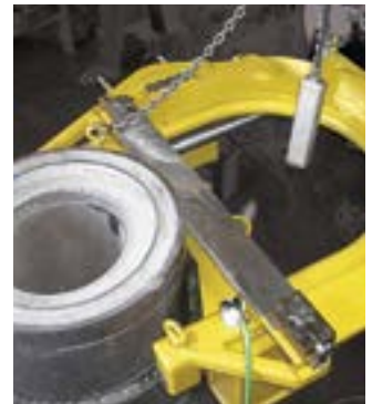
Goliath Saw shown on large diameter conductor
