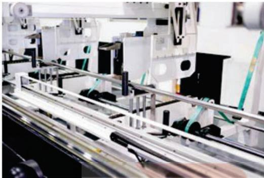
The loading system selects the tubes one by one and moves them to the measuring station;
