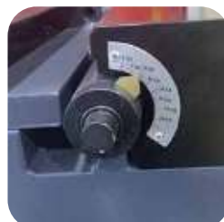
Easy Blade Gap Adjustment
