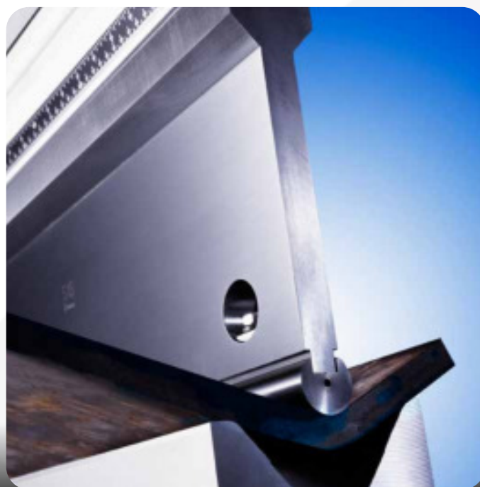
CUSTOM MADE TOOLS RADIUS HOLDER WITH INSERT
