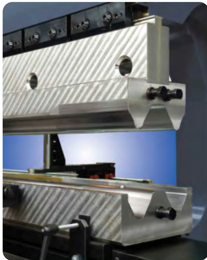
CUSTOM MADE TOOLS RADIUS HOLDER WITH INSERT
