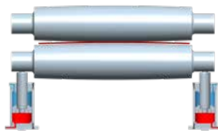
Bending thickness is thinner than roll crowning
