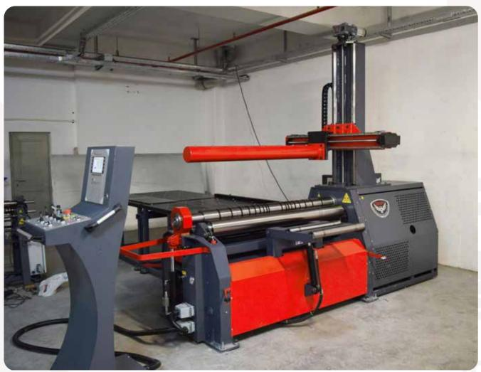
NC control system, in addition to the PLC control system, has the property to work manual, teach-in, and automatic modes of operation. In manual mode, the use of all functions are provided by the operator. In teaching mode for the operator to twist all the steps are recorded respectively. In automatic mode all recorded movements are repeated respectively by the machine.
