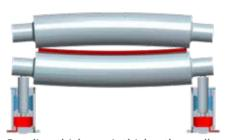
Bending thickness is thicker than roll crowning
