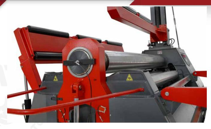
Hydraulic drop ends on RMT $^{\text{m}}$  Plate Rolls allow for easy removal of formed pieces. Also the top roll is hydraulically tilted up to allow for easy removal of formed parts. A roller type cone bending attachment is a standard feature that is placed on the lower roll housing. All RMT $^{\text{m}}$  plate rolls also include a safety wire surrounding the machine to automatically shut off the machine if necessary.
