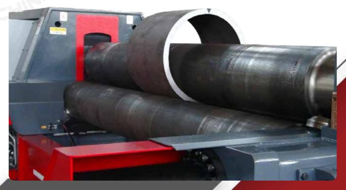
Another important feature of the R-HYBRID™ plate roll, is the press like system of the top forming roll. In fact, the top forming roll can be used as a traditional press allowing perfect re-rolling operation and calibration of thick plates. In the same way it is also possible to obtain cones with heavy thicknesses by bending the plate with several strokes.
