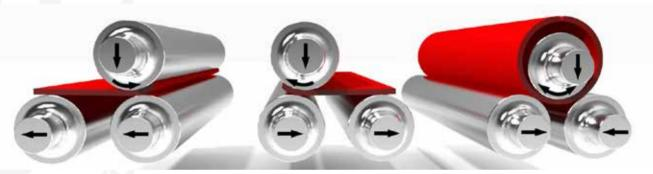
The pre-bending is performed by the top roll pushing directly against the first side of the plate, leaving a very short or null flat-end; the following rotation increases the curved initial side of the plate.
