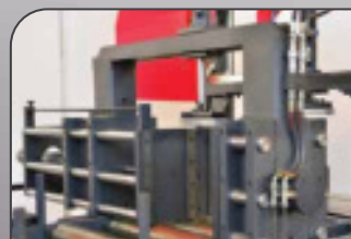
39- SERVO MOTOR FEEDING VICE 120" STROKE
