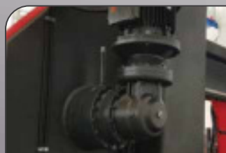
38- HEAVY DUTY PLANETARY GEARBOX
