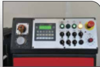
2- CONTROL PANEL NC
