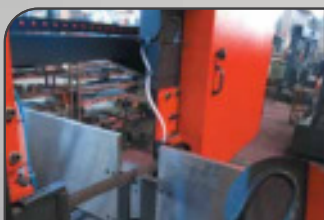
33- PROXIMITY SWITCH FOR SENSING BLADE SLIPPAGE
