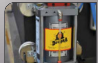
40- DROPSA AIR/ OIL CLEAN LUBRICATION SYSTEM
