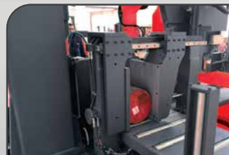
35- SERVO MOTOR FEEDING VICE 27" STROKE
