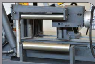
18- MECHANICAL TOP CLAMPING
