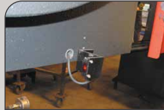
31- OPTICAL SAW HEIGHT ADJUSTMENT
