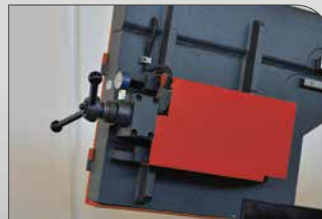
15- HYDROMECHANICAL BLADE TENSION
