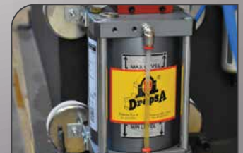
40- DROPSA AIR/ OIL CLEAN LUBRICATION SYSTEM
