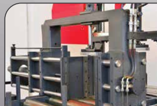
39- SERVO MOTOR FEEDING VICE 120" STROKE
