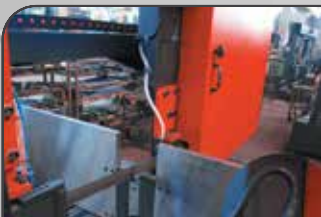
33- PROXIMITY SWITCH FOR SENSING BLADE SLIPPAGE
