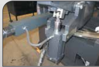
23- ANTI VIBRATION CYLINDER
